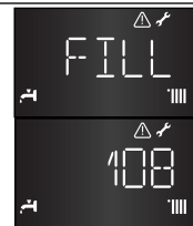
Figure 98 - Shut-Off Error for Low Water Pressure
