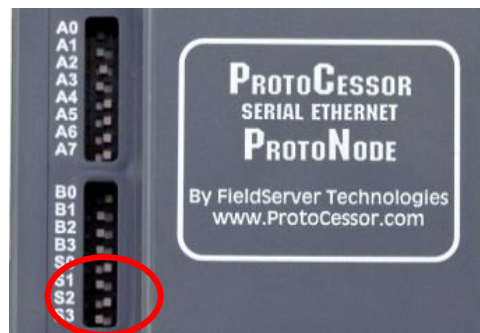
S Bank DIP Switch Location
