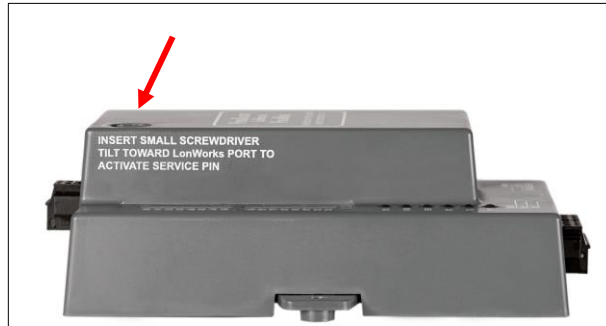
Figure 23: LonWorks Service Pin Location
