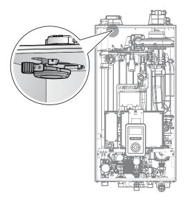
6. Remove the filter from the plastic assembly. Dust and rinse it with clean running water.
