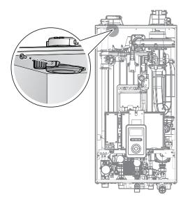
5. Pull the filter out of the boiler.
