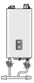
5. Remove the drain cap on the manifold system to drain the boiler.
