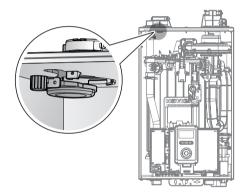
6. Remove the filter from the plastic assembly. Dust and rinse it with clean running water.
