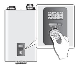
2. Press the Command dial ( ) to select the desired zone, and then press the Command dial ( ). The selected zone's temperature will flash.
