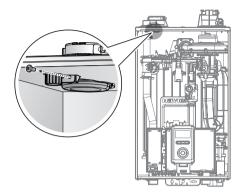
Pull the filter out of the boiler.
