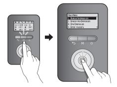
Rotate the Command dial ( ) to switch between the information items. Press the Command dial (🛞) to select an item and view the information.
