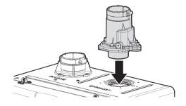
4. Tighten the four mounting screws to secure the Common Vent Collar Kit in place. The screws (x 4) are supplied with the Common Vent Collar Kit.
