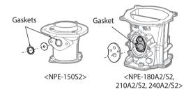
8. Replace the gas inlet pipe to its original position and use all screws to secure all connections.
