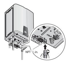
2. Place the free end of the drain line into an appropriate drain.
