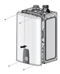
5. Loosen the screw indicated in the figure below and connect a manometer to the pressure port. Reset the manometer to zero before use.
