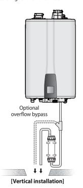
Ensure that the condensate runs freely to the drain.
