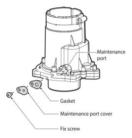
Through the maintenance port, check the operating condition of the damper plate inside the Common Vent Collar Kit.
