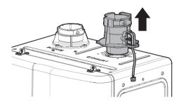
3. Connect the Common Vent Collar Kit to the exhaust duct of the water heater unit.
