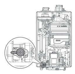
Press the Menu button (M) to access the Main menu and select 1. Recirculation Setting > 3. Internal Recirculation by pressing the OK button (OK).
