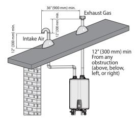
• Non-Concentric Sidewall Venting: Air is drawn from a different location that is at least 12 in. (300 mm) away from the exhaust termination. The exhaust termination can be located either on the sidewall or roof. Try to minimize the length of the intake air pipe when installing the vent.
