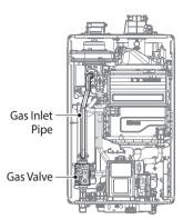
Figure 2. NPE-A2/S2 Series Internal Components
