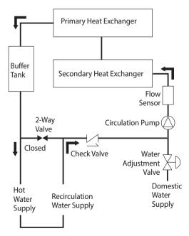
[External Recirculation Mode using the Recirculation Inlet]
